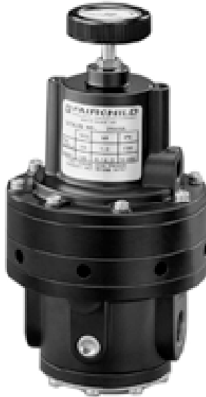
The Model 2500A Bias Reversing Relay provides an outlet pressure that decreases in direct proportion to increases in input signal.
